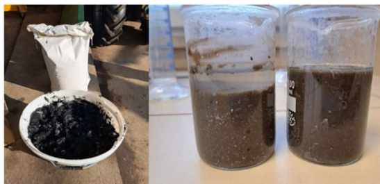
Fig 3. Stabilization of sludge with natural materials
